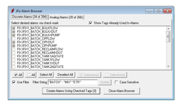
In the examples shown above, changing the wild-card from batch to "BATCH" - "MIX" "ETR" narrows the filtered list from 76 Discrete Alarms down to 34 (shown on the tab captions). The second list only shows alarms with "BATCH" in their name, but also excludes any alarms with "MIX" or "ETR".
