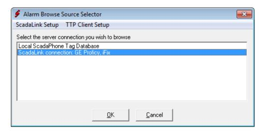
**Note**: Before proceeding, make sure to launch the iFix run-time environment so that ScadaPhone will be able to retrieve the tag information.
