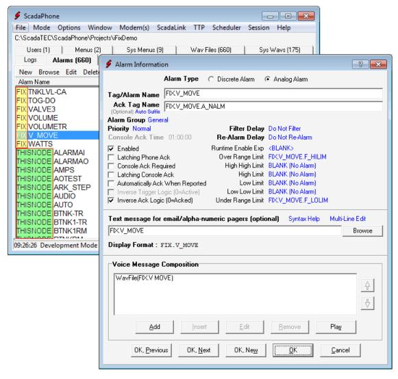
In this screen capture, note that the FIX.V\_MOVE alarm has been configured as an Analog Alarm with the following properties:
