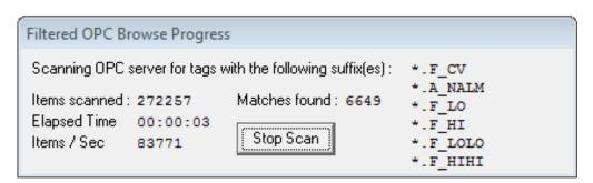
This window shows the progress of the iFix name-space browse. In this scan, ScadaPhone is compiling a list of all tags in the iFix project that have both \*.F\_CV and \*.A\_NALM suffixes: If a tag has an .A\_NALM suffix defined, it is assumed to be an alarm tag.
