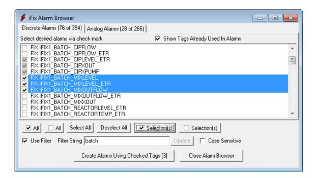
This window allows the user to select which tags from the OPC browse shall be configured as alarms in the ScadaPhone project. Note that the Analog Alarms and Discrete Alarms are segregated into two tabs and the selection list can be filtered to facilitate the selection process.
